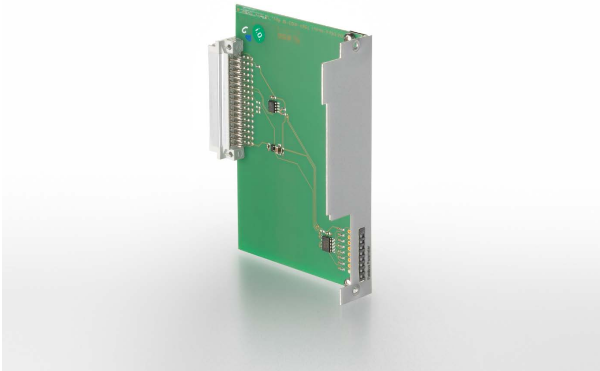
Figure 9: FBA module: Front view
