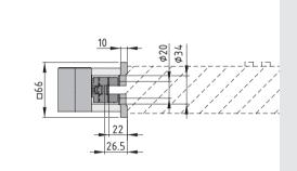
Clamping connection between motor shaft and coupling:
