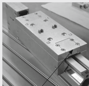
Timing Belt clamping device
