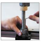
You will find it easier to fit the collet mechanisms if you first assemble the one at the floating bearing end. It is recommended that the fit of the collet in the bearing is checked prior to this and adjusted by relieving the bearing diameter if necessary with fine emery paper and a rotating mount. The fit of the collet in the bearing should be such that it can easily be removed axially using only gentle tabs with a hammer.
