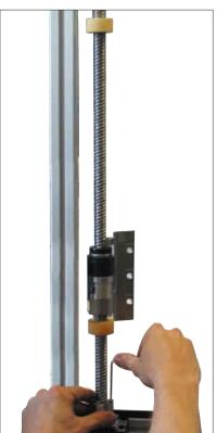
The spindle must be inserted vertically (eliminating any sag) into the collet mechanism, which in turn will be fitted into the floating bearing housing.
