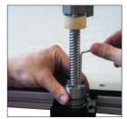
You will find it easier to fit the collet mechanisms if you first assemble the one at the floating bearing end. It is recommended that the fit of the collet in the bearing is checked prior to this and adjusted by relieving the bearing diameter if necessary with fine emery paper and a rotating mount. The fit of the collet in the bearing should be such that it can easily be removed axially using only gentle tabs with a hammer.
