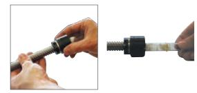
After the nut has been fitted, the gimbal adapter and yoke can be screwed on (to the flange side of the nut). To do this, the nut should be positioned carefully until its flange side is approximately 20 mm from the end of the spindle.
