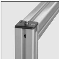
Integrated Lock System 8 is a modular Locking System for doors and flaps made with Line 8 Profiles. It is installed in the main Profile of the door frame („Door Profile“) and enables the door to be locked in up to three directions. Due to its modular design, the Lock System is suitable for locking doors whether they are left-hung or right-hung.
